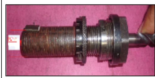
Holder to key face distance 17.7mm
